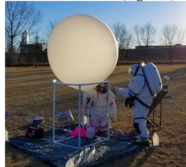
Figure 4: Fill tool updates, including balloon stabilization cage, enabling full crew autonomy during fill procedures.
