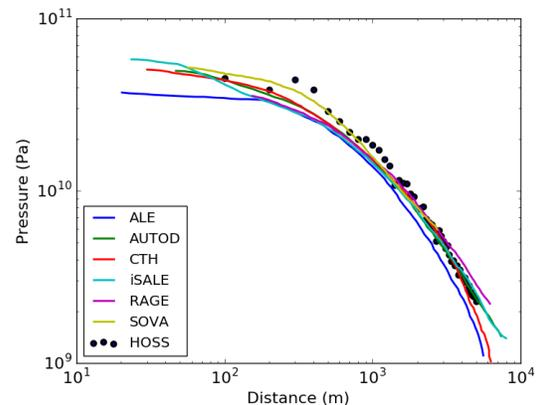
Figure 1: Pressure decay downward from the impact point of a 1km diameter aluminum sphere impacting an aluminum body. The results from HOSS are compared to a number of different numerical methods.
