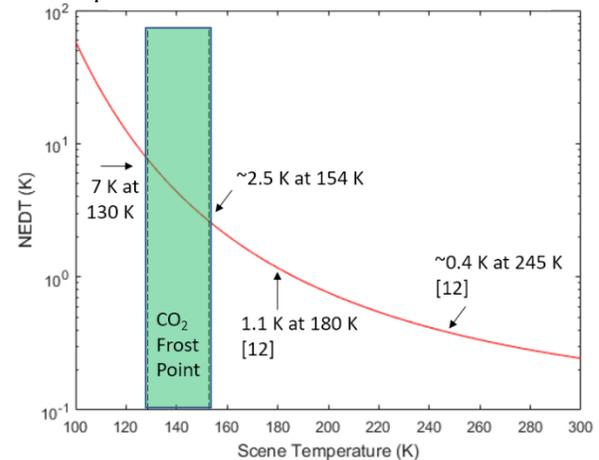
**Figure 1.** THEMIS band 9 Noise Equivalent Delta Temperature (NEDT) vs. scene temperature. The global temperature range of the CO<sub>2</sub> frost point is highlighted in green.
