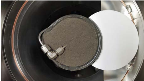
Figure 2. Top of the 50 cm JSC-1A simulant column with adjacent Spectralon® optical reference target for reflectance spectrometry.
