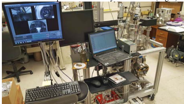
Figure 3. Data acquisition includes separate PCs and monitors for recording multiple camera views of simulant column (left) and mass spectra of the chamber interior (center).
