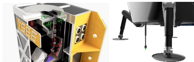
Figure 3: iSEE ConOps. iSEE illuminates a sample with a laser source to induce Raman scattering, and to collect and relay this light to a spectrometer where its intensity and distribution is measured, recorded, and analyzed in real time. (left) rover/lander delivers sample into iSEE viewport, where it is analyzed. (right) Spring-driven harpoon with a sensing head (viewport at its tip connected to a fiber optic). Sensing head pushed and held in place for surface analysis.
