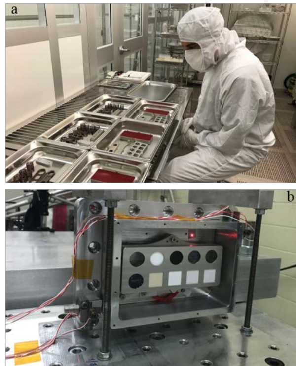
Figure 4: (a) final ultra-cleaning of SCT components in JSC Genesis Lab and (b) SCT shock testing setup.
