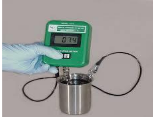
Figure 1. Example of a Model 1152 Digital Conductivity Meter used to measure the conductivity of a liquid.
