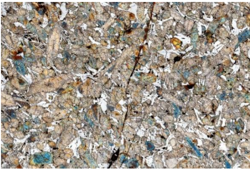
Figure 4. Partially cross-polarized light optical thin section image of NWA 12323. Maskelynite is white. Note the shock glass veinlet. Width = 18 mm.
