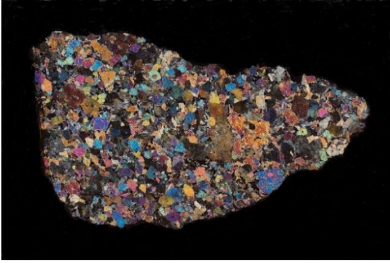
Figure 3. Cross-polarized light optical thin section image of NWA 11241. Width = 20 mm.
