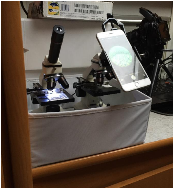
Figure 2. Microscopy setup with polarizing microscope (for geology experiments; left) and bright-field microscope with digital output (right) at the ExoHab, ESTEC.
