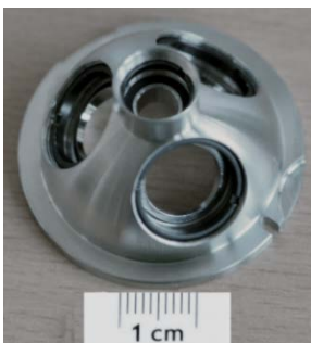
Fig. 3: Praying Mantis™ HighTemperature Reaction Chamber. Insert top left: Aluminum cup for mixed powdered fractions.
