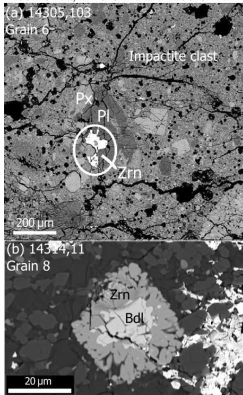
**Figure 1.** Backscattered Electron (BSE) images of (a) a poikilitic zircon grain, which is part of a mineral assemblage and located in an impactite clast, and (b) granular zircon surrounding a baddeleyite grain. Abbreviations: Zrn=zircon, Px=pyroxene, Pl=plagioclase, Bdl=baddeleyite.
