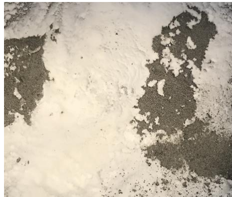
Figure 1: Simulated lunar ice formed by freezing gaseous ice components onto super-cooled lunar Highland regolith simulant before it is mixed in during the ice manufacturing process.
