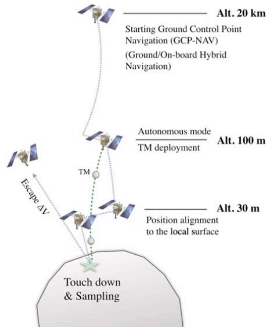
**Fig. 3.** Operation sequence for touchdown and sampling [1].
