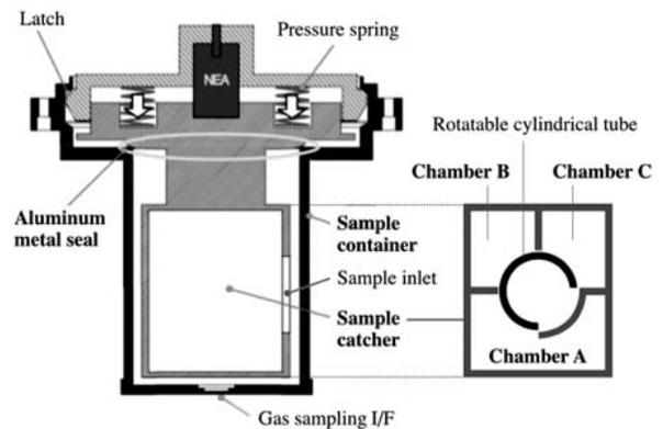
**Fig. 2.** Schematic illustration of the Hayabusa2 sample catcher and container [1].
