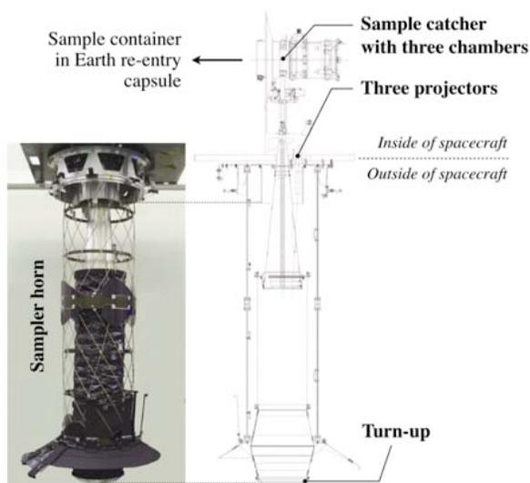
**Fig. 1.** Photograph of the Hayabusa2 sampler horn and schematic illustration of the Hayabusa2 sampler [1].
