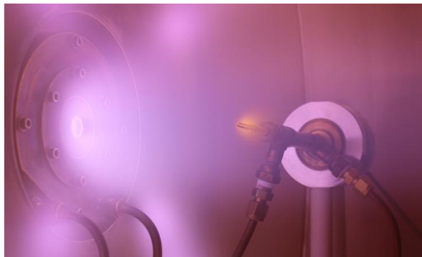
Figure 1: Electrostatic probe measurements in the IPG6-B facility during operation with argon
