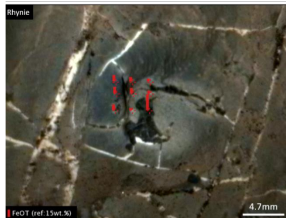
Fig. 1: Fe relative content (red lines) for each ChemCam sample location at the target Rhynie illustrating associations of high Fe with dark-toned features and of low Fe with bleached light-toned halos.
