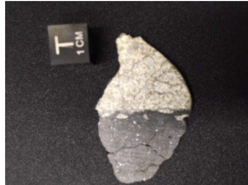
Figure 1: Sample of Chelyabinsk LL5 chondrite. Half of the sample is formed by a light (unaltered) lithology while the other half by shock-blackened/impact melt material.
