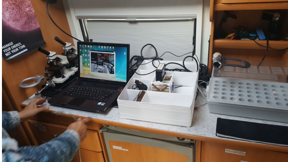
Figure 3. Prototype test bench in analog simulation habitat at ExoHab, ESTEC. Compact setup with microscopes, spectrometer, control computer and prototype astrobiology experiment. All can be stored in white boxes, displayed in middle of picture.
