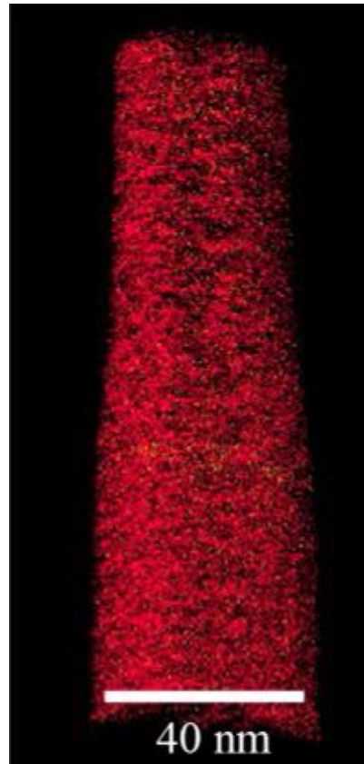
Figure 3. A 3 dimensional reconstruction of the atoms measured by atom probe analysis of the RMN in Figure 1 and 2. Each dot represents an individual atom detected during atom probe analysis. Re is represented by red dots and S by yellow dots. The sample is homogeneous with respect to its chemistry. This data set is typical for RMN in this study.
