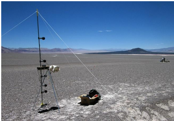
Figure 1. Context for the tower locations at CPP site, before commencement of data logging. Tower 1 (near field) is 2.8 m tall. Anemometer controllers were mounted on a tripod behind the tower. Note logarithmic height distribution of sensor heads. Tower 2 is about 50 m in the distance (at right).
