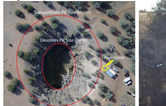
Figure 2. Left: Field test site. Red circles show size of terrestrial versus lunar pits compared to the Axel rover (yellow). Right: The Axel rover on a vertical basalt wall.
