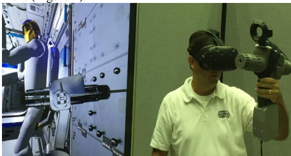
Figure 1: An example of the HR environment that SHyRE capitalizes on. Here, the user is able to see the ISS environment while also holding a physical copy of the tool he is using in the environment, the PGT. SHyRE will build on this by creating a scientifically relevant environment and making handheld scientific instruments available to the user.
