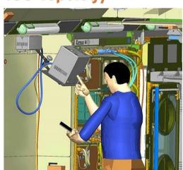
Mochii will be aisle-deployed in the Japanese Experiment Module (JEM) and will be powered by 120VAC inverter (95th percentile male shown, see also center image in banner above).
