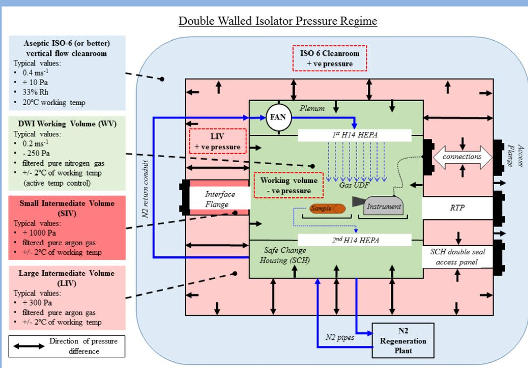
Figure 2. Double Walled Isolator Pressure Regime & System Overview.
