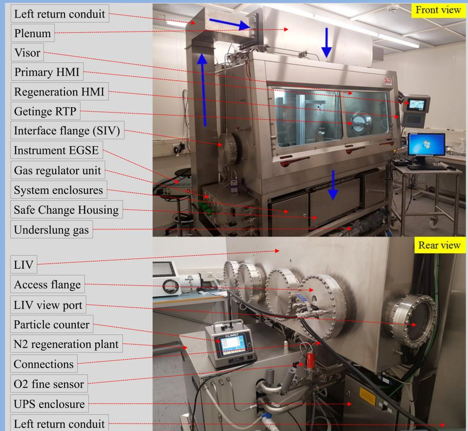
Figure 1. Double Walled Isolator Breadboard at the Class 1000 Aseptically Managed Planetary cleanroom of the University of Leicester. The DWI is c. 2.4 m wide & 1500 kg.
