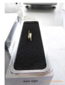
Thermal conductivity of the UTPS-TB is low even for the bulk material and  $< 0.1 \text{ W m}^{-1} \text{ K}^{-1}$  between  $-150^\circ \text{C}$  and  $+50^\circ \text{C}$ . This is likely due to the significant micro-porosity.
