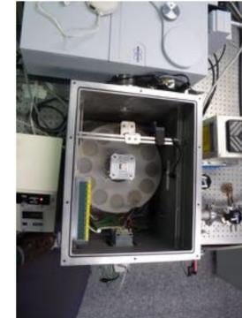
Instrument Bruker Vertex 80V (under vacuum) coupled via a shutter with evacuated emissivity chamber containing blackbody, stepper motor, sample holding carousel, webcam, and an induction system to heat the samples from 320K to above 900K. Complementary reflectance and transmission measurements via dedicated hardware units in 0.4 to 200  $\mu\text{m}$  spectral range.
