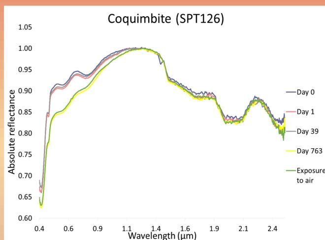
Figure 1: Coquimbite (SPT126) reflectance spectra (with sapphire window)
