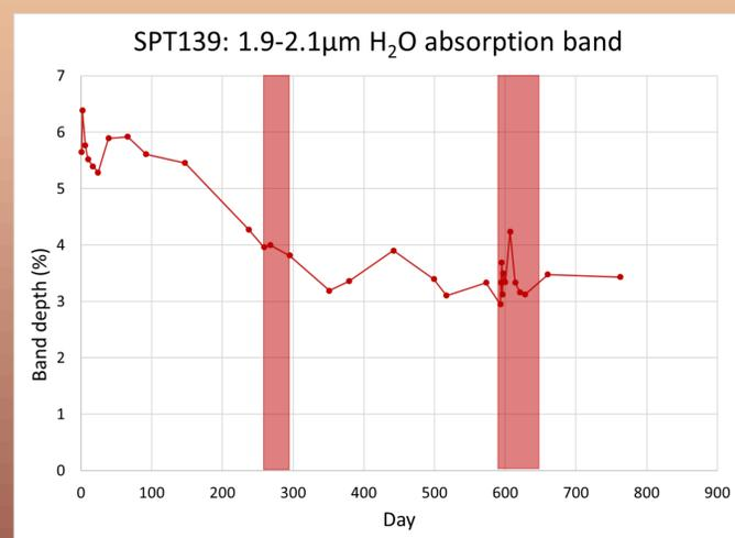
Figure 3: SPT139 Rhomboclase band depth (%) over time (763 days) for the H<sub>2</sub>O 1.9-2.1 μm band with two periods of ultraviolet (UV) light irradiation
