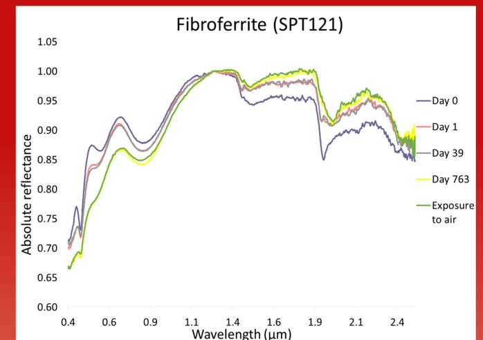
Figure 4: Fibroferrite (SPT121) reflectance spectra (with sapphire window)
