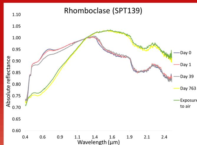
Figure 2: Rhomboclase (SPT139) reflectance spectra (with sapphire window)
