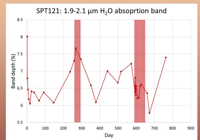
Figure 5: SPT121 Fibroferrite band depth (%) over time (763 days) for the H<sub>2</sub>O 1.9-2.1 μm band with two periods of ultraviolet (UV) light irradiation
