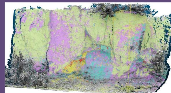
A multi-spectral imaging spectrometer (~800 to 2500 nm) to measure spectral reflectance to interpret the surrounding mineralogy, and identify targets of interest.
