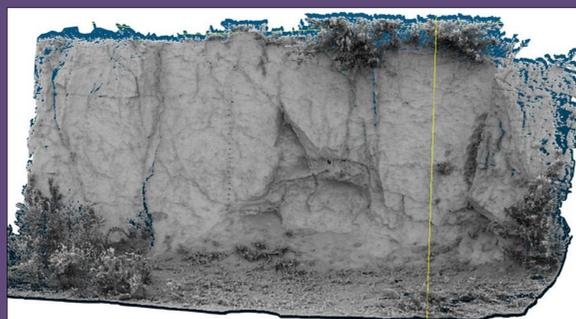
A Light Detecting and Ranging sensor to model the surface environment, analyze the topography, produce a hazard map for future human activity, and map the surface terrain to understand its formation.
