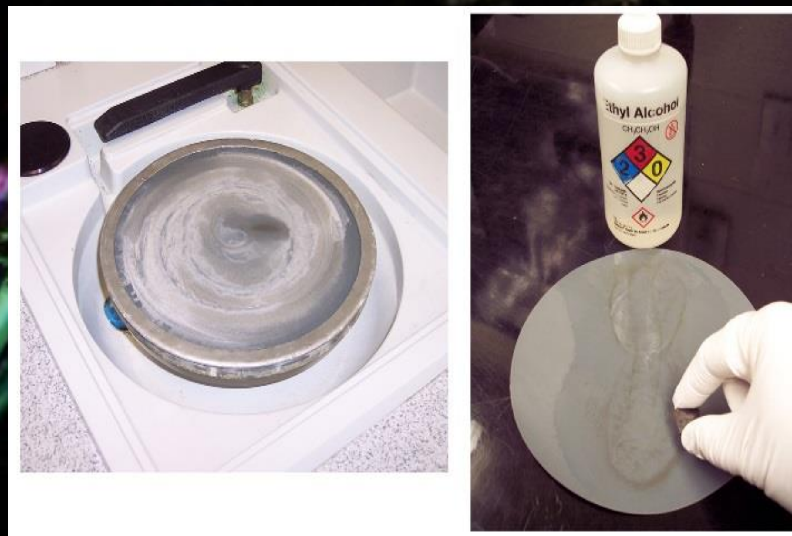
Fig. 2 – Powered lap wheel vs hand lapping. (NASA JSC)
