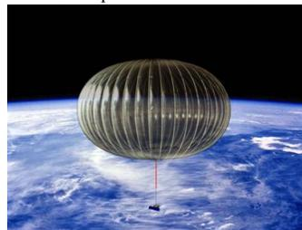
An example of a NASA high altitude balloon. CARDINAL will fly as a "piggy back" payload for high altitude (up to 36.5 km), low-air-speed CD particle collection.
