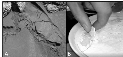
Fig. 1. A: 2-3 cm thick duricrust layer, Gusev Crater. Image 2P169853678EFFAAE0P2422L7M1. B: Duricrust simulant produced using Ottawa sand and sulfate salts; 3 mm thick.
