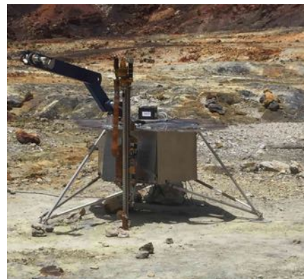
Fig. 2. ARADS drill tested with SOLID instrument (black case) and sample transfer arm at Rio Tinto in June 2017.
