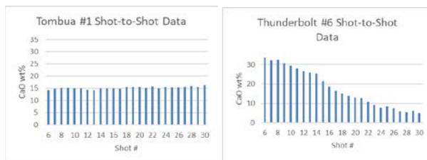
**Fig. 3** A. ChemCam shot-to-shot data for target depicting homogeneous calcium sulfate cement, Sol 1378. B. ChemCam shot-to-shot data displaying heterogeneous trend caused by hitting the edge of a vein, Sol 1033.
