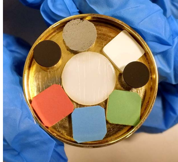
Fig. 3. Samples under analysis on the PASC chamber, including two options for black samples, an organic epoxy, a piece of PET and the RGB plus white samples
