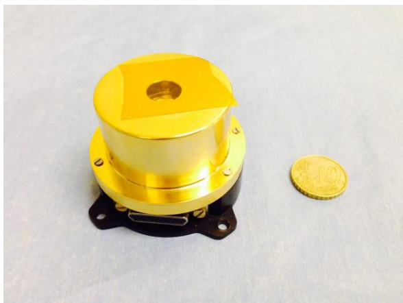
Fig.1. VISTA SH1 Engineering Model, i.e. Quartz Crystal Microbalances -based instrument.
