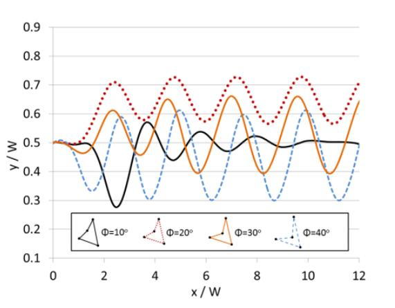
Fig 2. Settling trajectories of boomerang particles of different concavities. The surface area of the particles are the same. [5]
