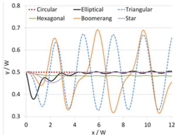
Fig 1. Settling trajectories of particles with different geometrical shapes [5].
