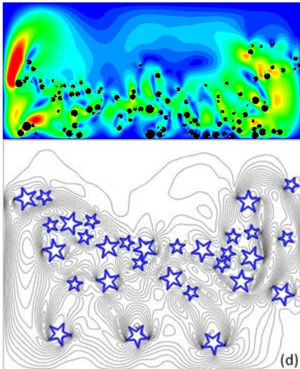
Fig 3. Gravity-driven settling ( $9.81 \text{ m/s}^2$ ) of 30 circular-shaped (top) and 30 star-shaped (bottom) particles in initially quiescent water. [5]
