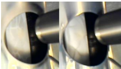
Figure 4: Visual examples inside the simulation chamber of ice mixtures condensing onto the cold head
