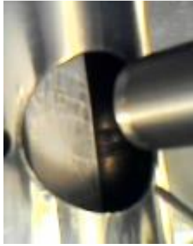
Figure 2: Visual example inside the Pluto simulation chamber of 5% carbon monoxide, 95% nitrogen at 10 K and 14 microbar pressure. FTIR probe on right.
