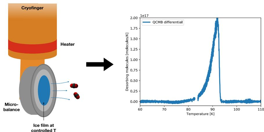
**Figure 1:** (left) Cartoon of the experimental setup with a desorbing ice film on a microbalance attached to a cryocooler. (right) Pure CO<sub>2</sub> ice sublimation rate as a function of temperature.
