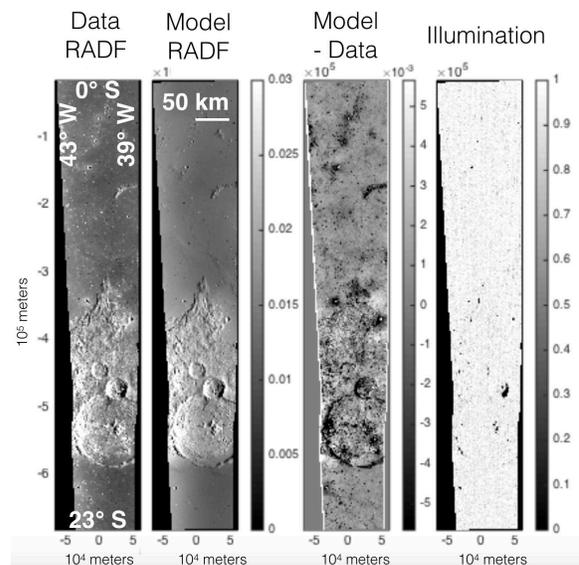
**Figure 1.** Modeling of a 566-nm WAC observation using the LOLA 64ppd map and the Hapke photometric parameters from [13].
