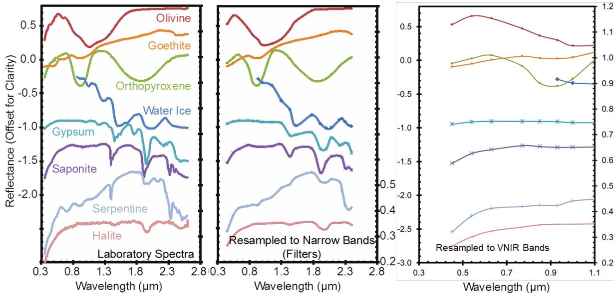
**Figure 1.** Laboratory spectra of minerals relevant to planetary surfaces (Left) convolved to AMIM's narrow band-passes (Middle) and an instrument with bands in the VNIR range (Right). Minerals have been offset for clarity; Serpentine and Halite values are on the right, others are on the left. AMIM's bands (Middle) enable the instrument to discriminate both iron and non-iron bearing mineralogies with greater fidelity compared to an instrument with bands in the VNIR range (Right).
