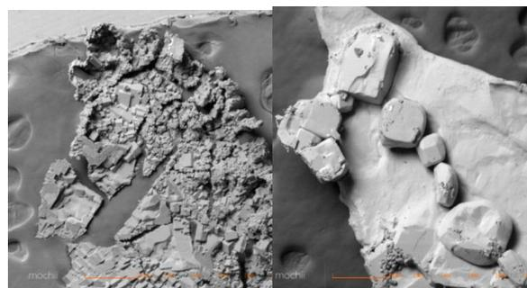
**Figure 4.** (left) NaCl polycrystals formed in earth gravity by evaporation, and (right) large single crystals of NaCl formed in microgravity by evaporation, both imaged in Mochii at same magnification. A small number of nucleation sites form large stable monolithic crystals in microgravity.
