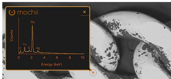
**Figure 2.** Energy-dispersive X-ray (EDS) spectrum acquired with Mochii S on gold alloy.
