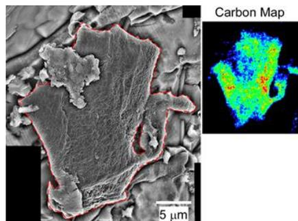
**Figure 3.** Left: SEM image of carbonaceous matter on freshly fractured surface of the Mars meteorite Nakhla. Right: EDS carbon map of the region outlined by the red dashed line in left image.
