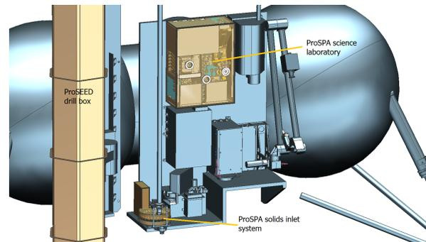
Figure 1: ProSEED and ProSPA Elements of PROSPECT on board Luna 27 platform.
