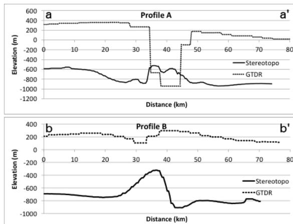
Figure 3. Topographic profiles sections a and b, showing a comparison between Magellan GTDR and stereo-derived topography. Vertical exaggeration =  $\sim 25 \times$ .
