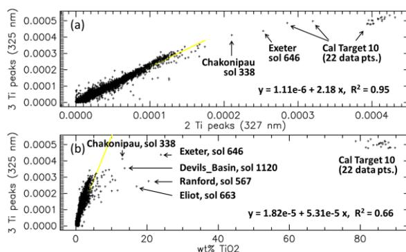
**Figure 3** Analysis of Ti-peak areas obtained from fitting of Cu/Ti bands (see Figure 2). The sum of 3 peak areas (left band) is plotted against the sum of 2 peak areas (right band, [a]) and against standard ChemCam MOC abundances [b].
