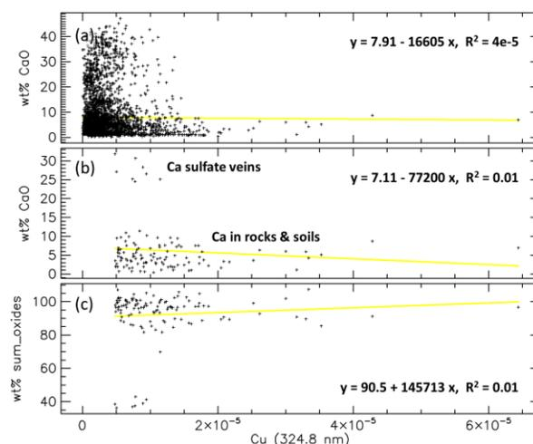
**Figure 6** (a) CaO abundance (wt%) plotted against left-Cu peak area (324.8 nm) for 3670 averaged ChemCam spectra (same selection as in Figure 4b). (b) Same as (a), but only plotting 119 data points (strongest Cu targets as in Figures 4c and 5). (c) Same as (b), but plotting the sum of (refractory) oxides on the y-axis. The rocks & soils from (b) now plot in the region near 100 %, while the veins host a “missing component” ( $SO_3$ ,  $H_2O$  and maybe other volatiles).
