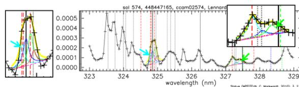
**Figure 2** Fit example according to model in Table 1. Cu lines are marked by teal (left band) and green arrow (right band). Vertical lines as in Figure 1. Fit codes use software by C. B. Markwardt, GSFC, USA (<http://purl.com/net/mpfit>).
