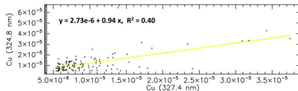
**Figure 5** Correlation between left and right Cu line for 119 ChemCam targets with strongest Cu signal (see Figure 4c). The slope is close to one in agreement with NIST’s assertion that both Cu lines do have same “relative intensity”.
