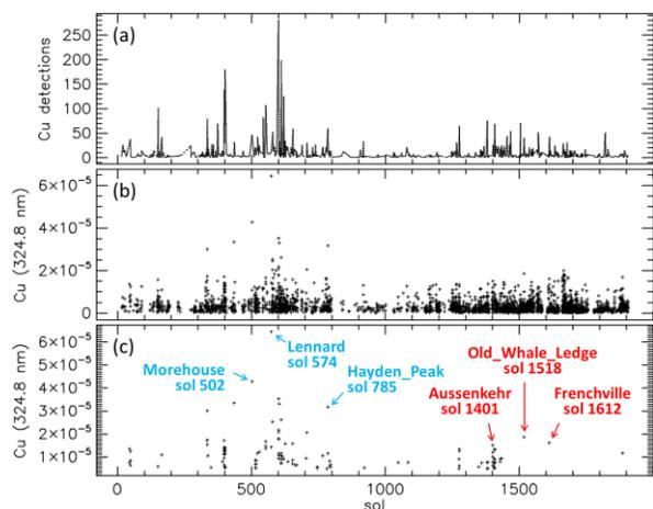
**Figure 4** Detection of Cu along the rover traverse. (a) Number of Cu detections. (b) Peak areas extracted from 3670 averaged spectra. (c) Same as (b), but making an even stronger selection (119 top-5% strongest Cu peak areas). A peak area of  $6 \cdot 10^{-5}$  may correspond to ~1000 ppm [3].
