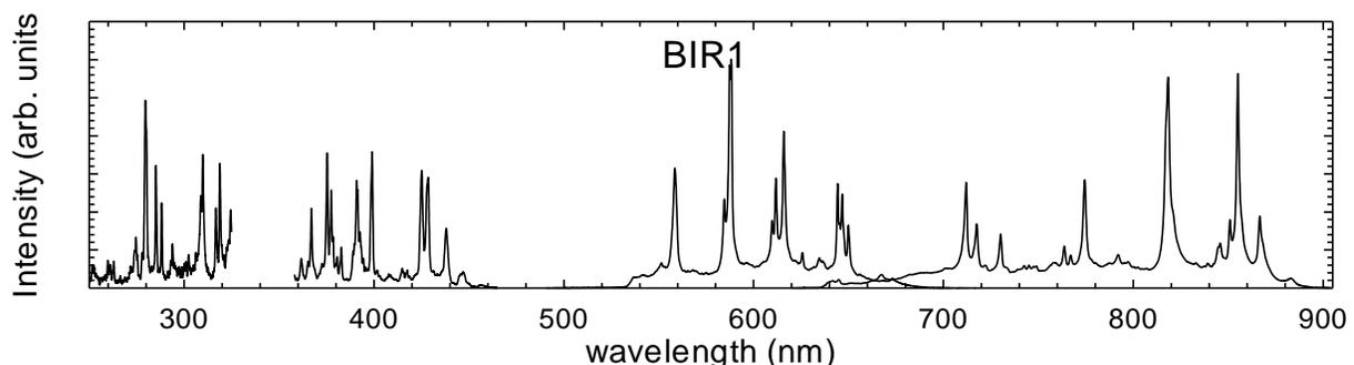
**Figure 1:** LIBS spectrum of the Islandic River Basalt (BIR-1) under simulated Venus atmospheric temperatures (465°C) and pressure (92 atm).
