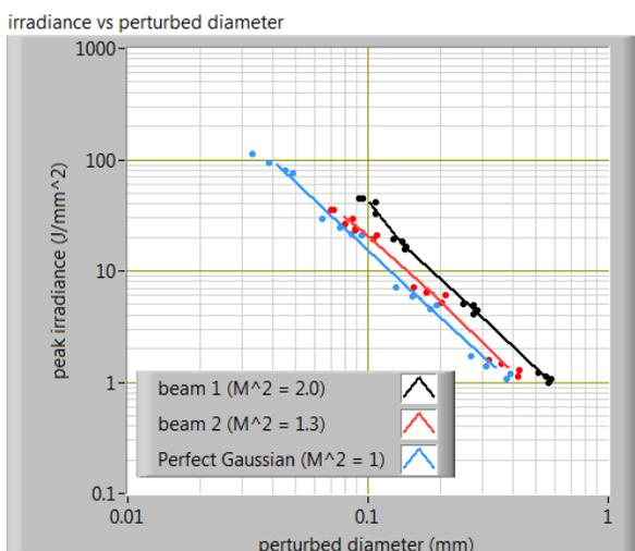
**Figure 3:** Changes in irradiance as a function of beam quality and distance. These results demonstrate that changes in irradiance due to turbulence are minimal.
