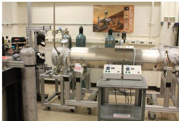
**Figure 4.** The 2 m long, 110 mm diameter Venus chamber capable of storing >92 atm of CO<sub>2</sub> at >465°C.
