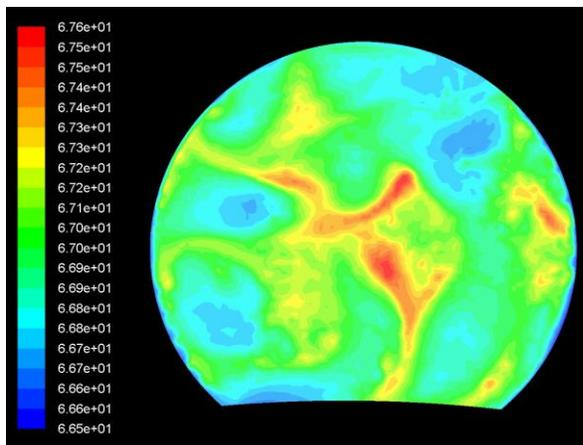
**Figure 2:** Contours of fluid density on the window. For reference, the window is approximately 87 mm in diameter. These contours represent only a **1.6%** change in density.
