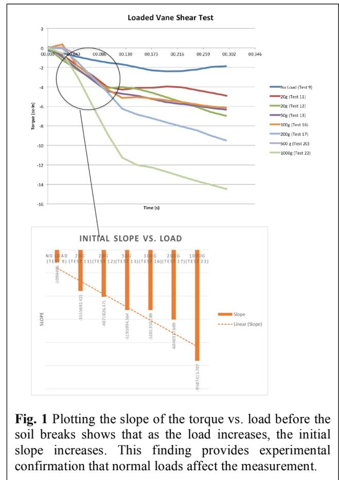
**Fig. 1** Plotting the slope of the torque vs. load before the soil breaks shows that as the load increases, the initial slope increases. This finding provides experimental confirmation that normal loads affect the measurement.
