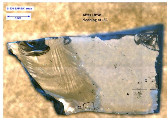
Fig. 1. Genesis sapphire sample 61530 after UPW cleaning at JSC. Most SEM studies focused on areas C1 (bottom) and D (right).
