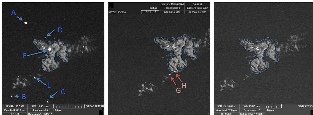
Fig. 2. BSE image of area C1e of 61530, before (left), after  $\text{HNO}_3$  (middle) and  $\text{NH}_4\text{OH}$  leach (right). FOV in each image is 65  $\mu\text{m}$ . Particles A-E were removed during  $\text{HNO}_3$  leach, while particle F was reduced in size, and G and H were redeposited. An outline of the main Si contaminant is shown before cleaning and copied to each image
