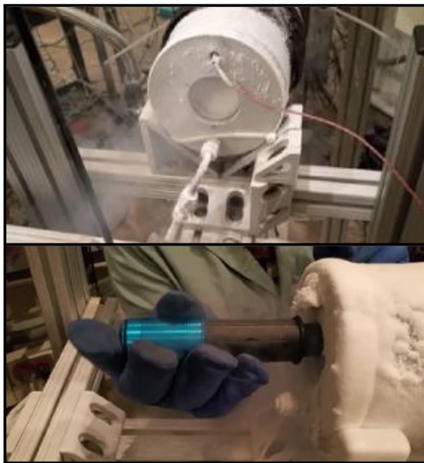
Figure 2. Top: Photograph of the ice radiation chamber, held at ~88 K by constant flow of LN 2 . Bottom: Testing surface roughness following bombardment of the ice surface with 10.5-25 MeV electrons at a total dose of \sim 8 \times 10^{16} MeV cm -2 .
