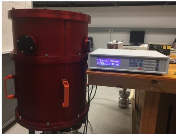
**Figure 2.** Vacuum chamber with cold plate (left) with controlling electronics (right).
