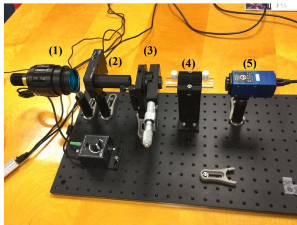
**Figure 1.** Experimental set-up. Components are (1) LED light source; (2) collimator optics and polarizer; (3) Soleil-Babinet compensator (for calibration); (4) cylindrical sample cuvette; (5) polarization imager camera.
