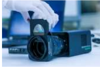
Fig. 1. (a) Photo of a transmitted diffraction grating of METEOR. (b) Photo of (a) manually installed in the built-in slot of METEOR lens.
