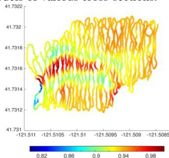
**Figure 4:** Magnetic survey of Skull Cave normalized to maximum recorded value. In this example, the lava tube is revealed as a magnetic high [10].
