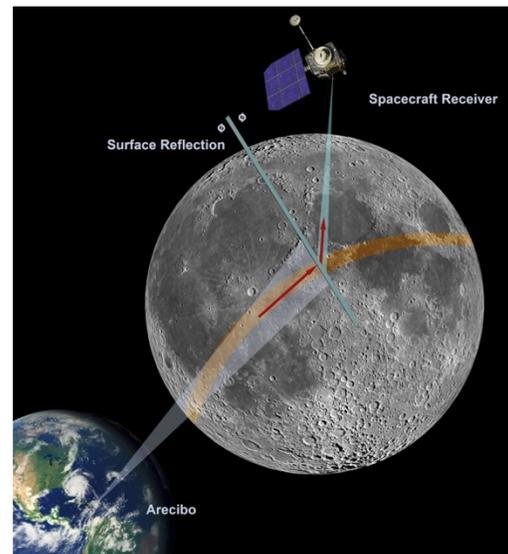
**Fig. 1:** An illustration of the forward scattering observation geometry where the incidence and emission angles were identical. Mini-RF has obtained one such observation, to date, for a location near the center of the Aristarchus pyroclastic deposit. These data can be modeled to derive the permittivity at the target region. Credit: NASA GSFC/J. Friedlander.
